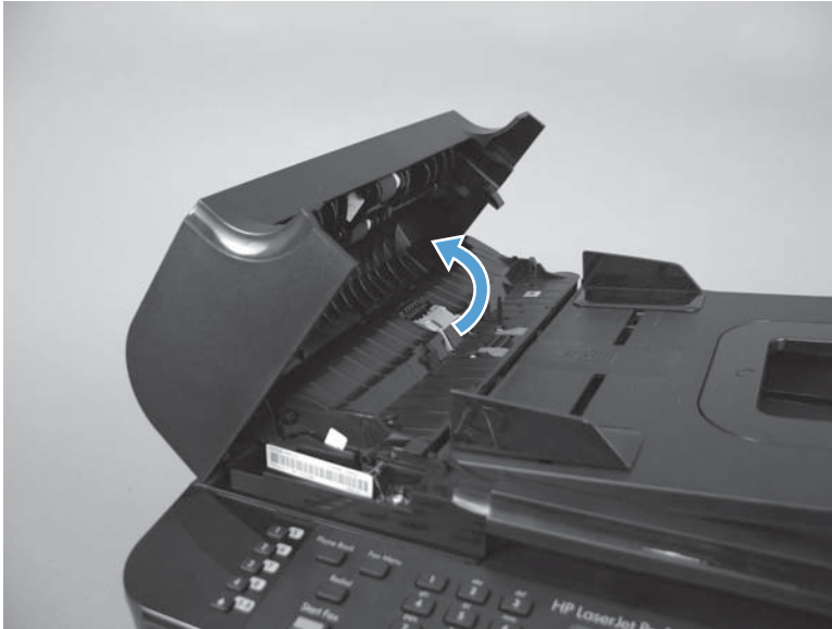
Figure 1-121 Remove the document feeder cover (1 of 3)
