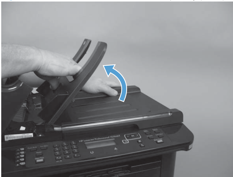
Figure 1-120 Remove the document feeder input tray (2 of 2)
