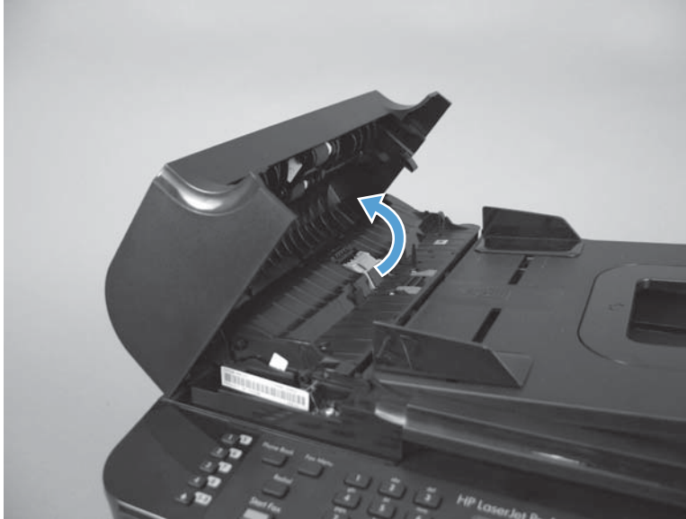
Figure 1-119 Remove the document feeder input tray (1 of 2)
